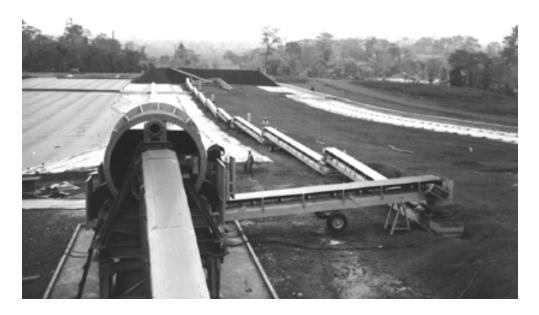
**Figure 6** Agglomerating drum and conveyor stacking system with 6 meter high heap at Ity, Ivory Coast.
