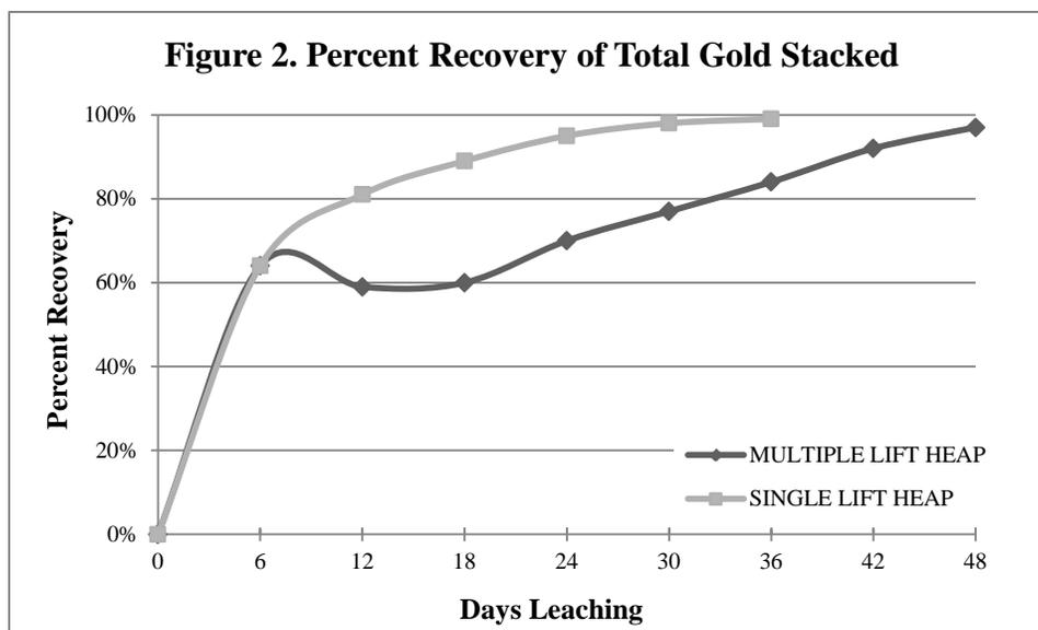
Figure 2, above, reproduces the single-lift curve from Figure 1, but adds a second curve which is a typical curve for percent recovery of gold stacked on a multiple-lift heap. The upper curve is the single-lift heap. The lower multiple-lift curve takes a dip late in year one, as it assumes that the second lift began after six months.
