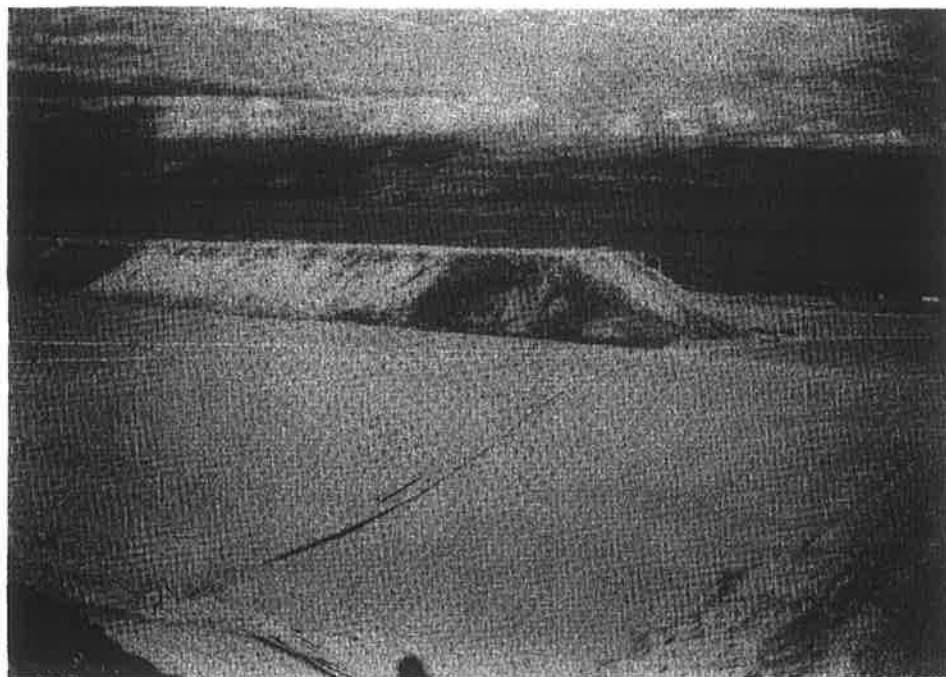
Figure 9. Heaps of 12,000 tons each are built, 15 feet high, atop gravel-covered PVC pads. Lots of land is available on the alluvial fan below the mine.
